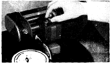
Fig. 5-25. Angle and depth of cut are controlled by these two knobs atop the carriage.
