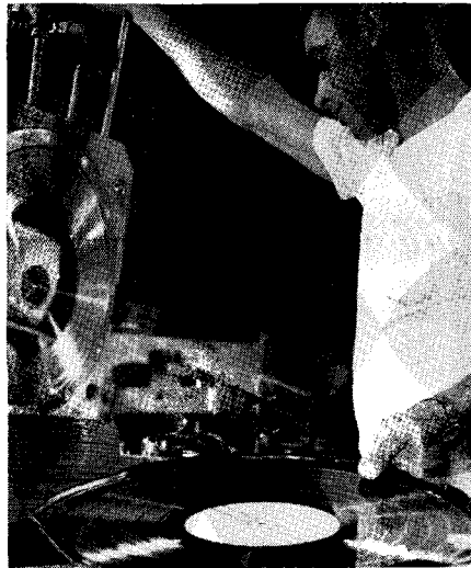
Fig. 27-15. The transcription as it comes from the die of record stamping machine.
