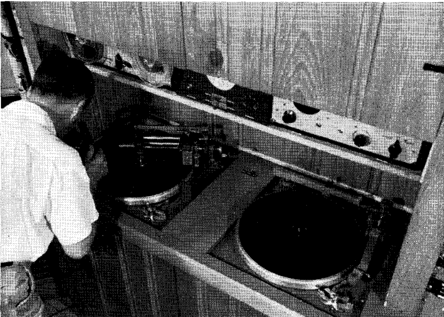
Fig. 26-5. Birds-eye view of the turntable console, showing two Presto 6N tables. (Courtesy RADIO & TELEVISION NEWS)
