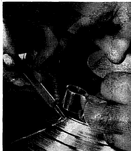
Fig. 27-10. Craftsman repairing a defective groove on the metal "mother."
