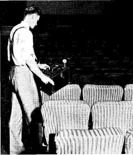
The General Radio type 759-B sound level meter being used to perform acoustic measurements in a motion picture theater.
