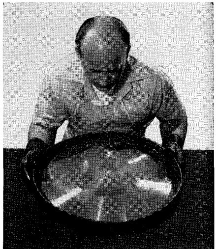
Fig. 27-1. Silverplating the "master" recording.
