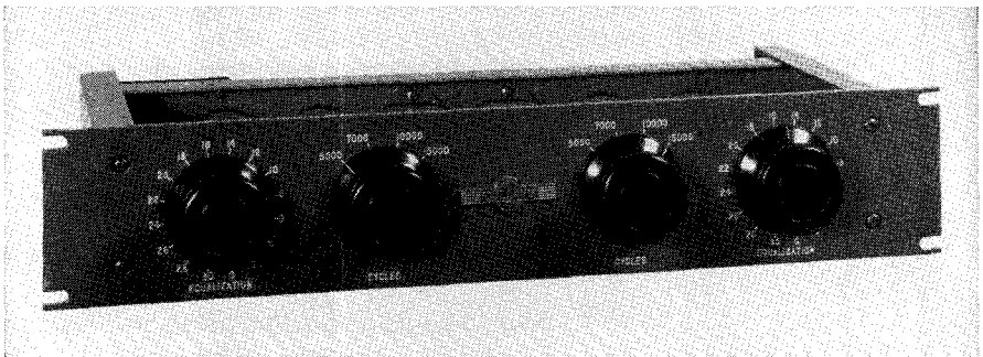
Fig. 17-33. Collins 116E-4 program equalizer. (Courtesy Collins)
