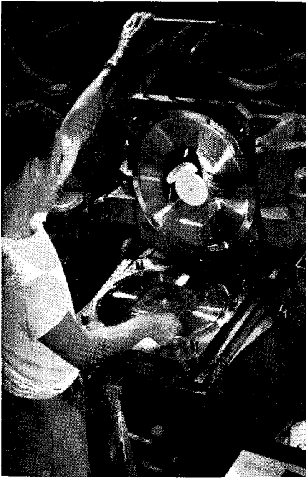
Fig. 27-14. The heat and high pressure of the stamping machine form the transcription from either special plastic or shellac material.
